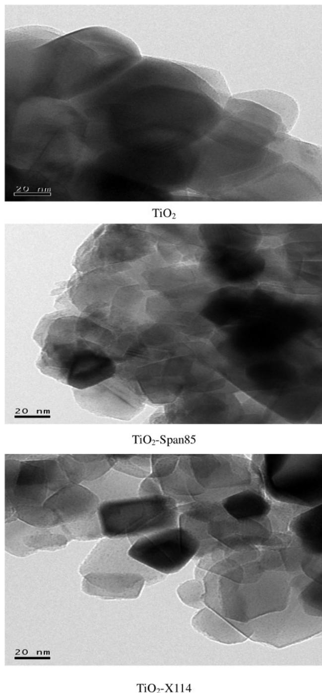
**Figure 5.** TEM images of  $\text{TiO}_2$ -X114,  $\text{TiO}_2$ -Span85 and  $\text{TiO}_2$ .
