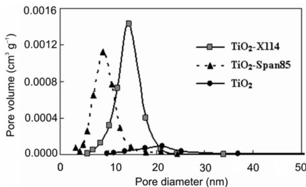
**Figure 3.** Pore size distributions of  $\text{TiO}_2$ -X114,  $\text{TiO}_2$ -Span85 and  $\text{TiO}_2$  derived from desorption branches of  $\text{N}_2$  adsorption/desorption isotherms.
