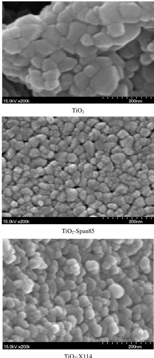
**Figure 6.** SEM images of  $\text{TiO}_2$ -X114,  $\text{TiO}_2$ -Span85 and  $\text{TiO}_2$ .
