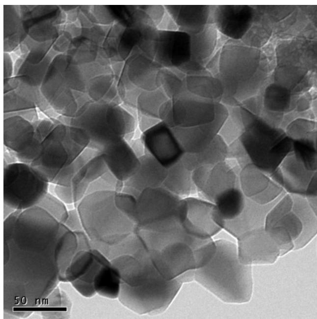
**Figure 4.** TEM image of sample  $\text{TiO}_2$ -X114.
